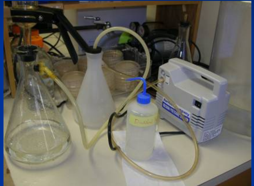
Filtration system to wash the algaecides from the spores
