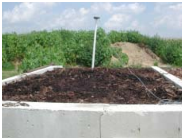
133 Figure 1. Relative humidity sensor with extension tube in biofilter medium, field trial.
